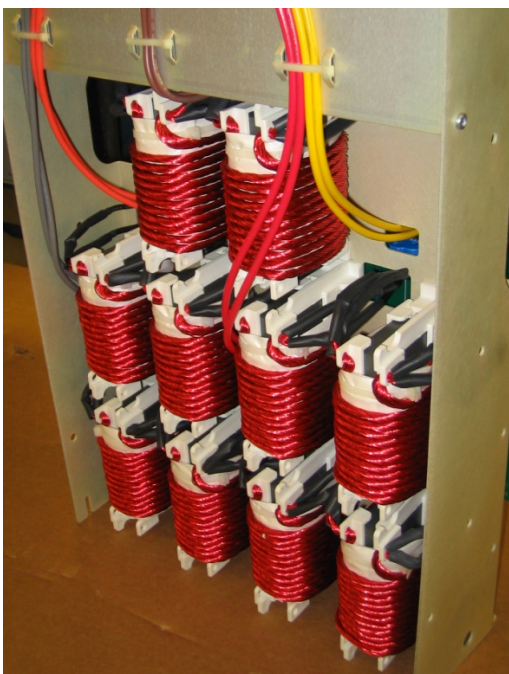
Picture 2. Inductors for half of a complete powertrain of the transformer-free topology
